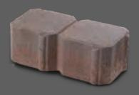
FULL BRICK 4-1/2" x 9" x 3-1/8" .272 sq. ft. per unit 3.68 units per sq. ft. 36 units/layer, 252/cube HALF BRICK 4-1/2" x 4-1/2" x 3-1/8" .136 sq. ft. per unit 7.35 units per sq. ft. 8 units/layer, 56/cube
